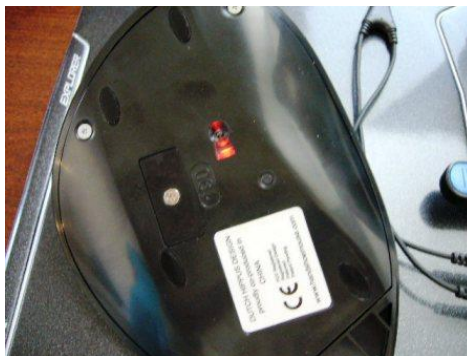
Battery is charged, red light is on
