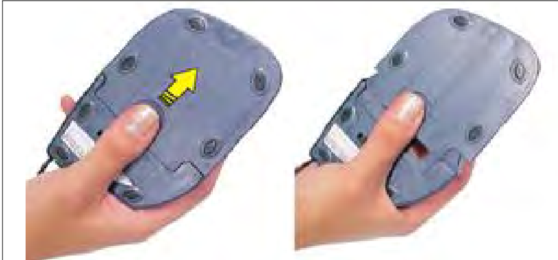
Fig. 5. – To change palm of the hand adapters, press and push forward as indicated.
